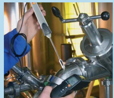
Connection for external temperature probes (testo 830-T2/T3)
